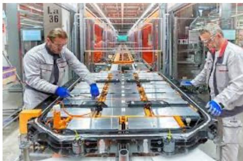
A typical EV battery weighs 450 kilograms. It contains 11 kilos of lithium, 27 kilos of nickel, 20 kilos of manganese, nearly 14 kilos of cobalt, 90 kilos of copper, and 180 kilos of aluminium, steel, and plastic. Inside are over 6,000 individual lithium-ion cells. All those toxic components come from mining. To manufacture each EV car battery, you must process 11,000 kilos of brine
